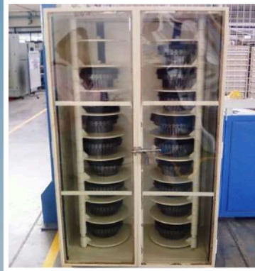
Cutter Storage Rack for Gear Plant
